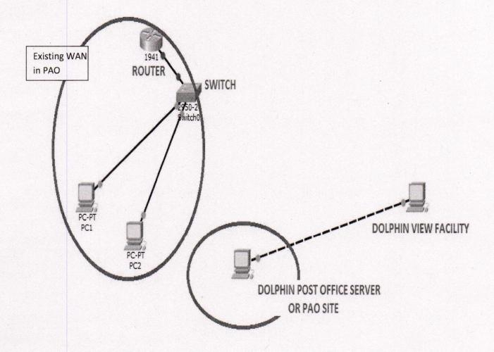
(ii) Step-I: Using 8-port switch connect the already one to one connected PCs through WAN.
